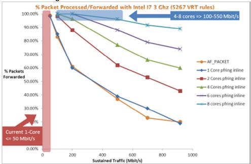
This graph again illustrates that using Pfring inline to parallelize the inline processing increases performance with the VRT rules as well.
